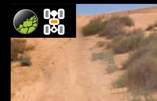
4LLC (4WD Low Range with locked centre differential) For steep hills, sand, deep snow, etc. ^
